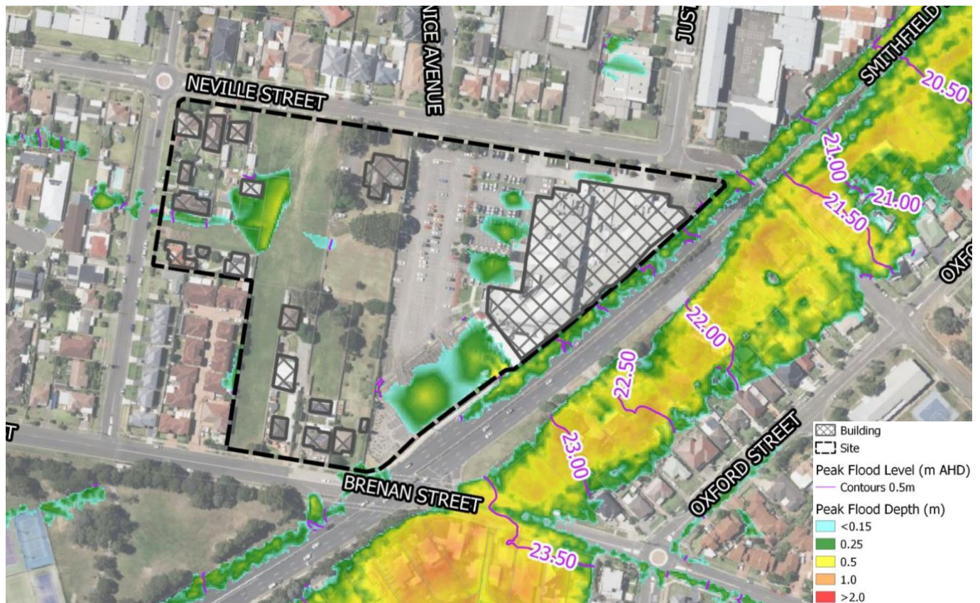
Figure 4-2 Existing conditions flood depth results (1% AEP) (BMT WBM, 2024)
