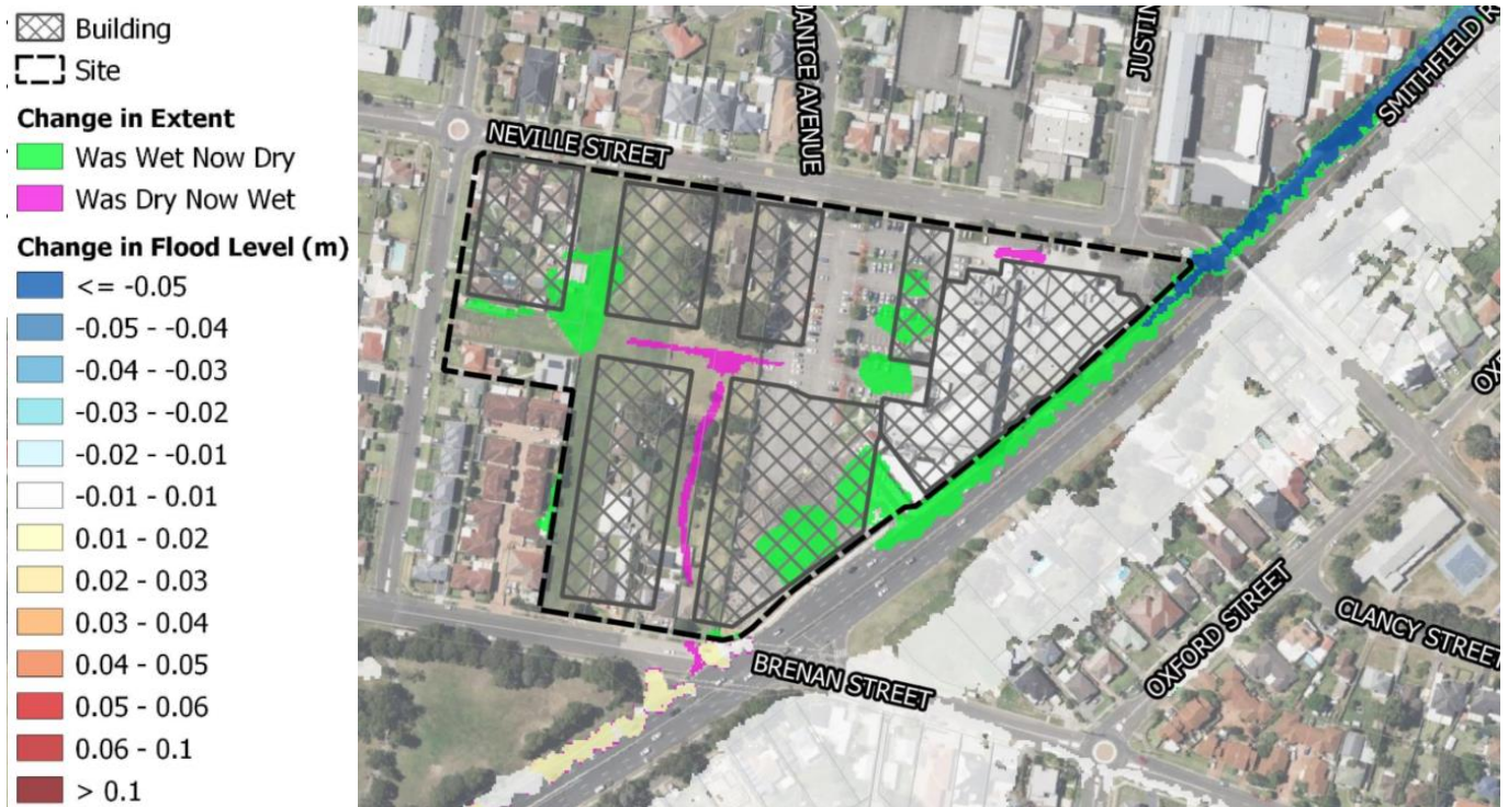
Figure 4-4 Flood Afflux results (1% AEP) (BMT WBM, 2024)
